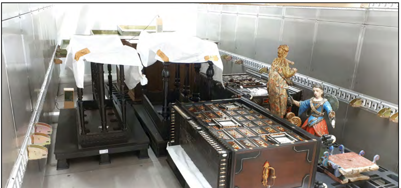
The 40 m 3 ICM chamber in Brussels. Treatment of two insect-infested Flemish cabinets, wood veneered with tortoiseshell, inlaid and solid ivory, fire-gilded brass fittings. Next to it two painted sculptures. Photo: ICM Europe, Kampenhout
