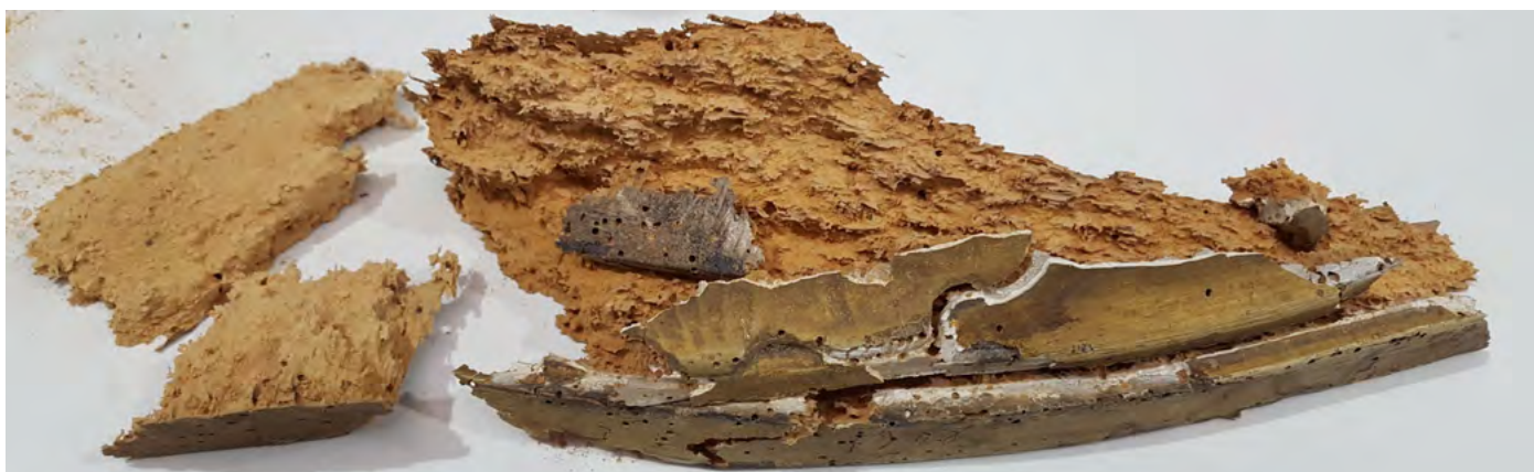
Drastic loss of substance by Anobium punctatum infestation, parts of a polychrome procession throne, 19 th cent. Photo: ICM Europe
