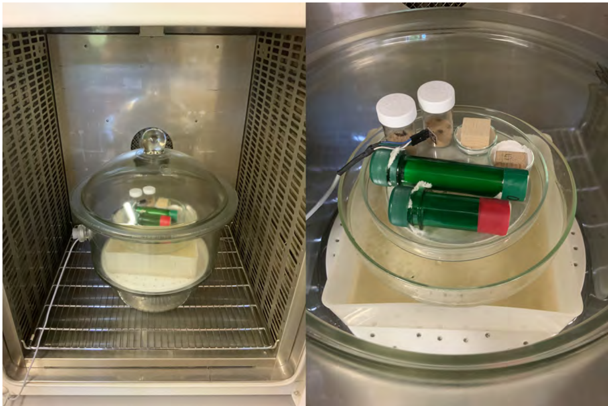
Part of the experimental setup for lethal temperature determination for Anobium punctatum , Lyctus brunneus , Ctenolepisma longicaudatum and Tineola bisselliella . Left: Heating cabinet with exsiccator. Right: the insect samples in plastic containers. Photo: ICM Europe
